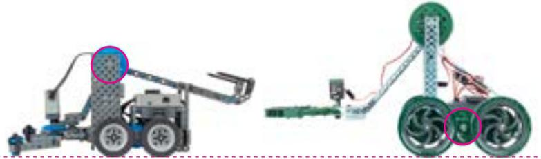
Some VEX IQ and VEX EDR gears are the same diameter and tooth count. In this instance, matching the scale of the 60 Tooth gear between the two Clawbots was the best choice.
